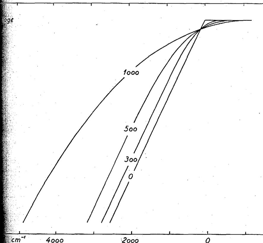
Fig. 23. Theoretical curves for  $\log \epsilon = \log G$  calculated for  $T = 298^\circ K$  and for different values of  $\sigma$  as indicated. The ordinate is given in logarithmic units.
