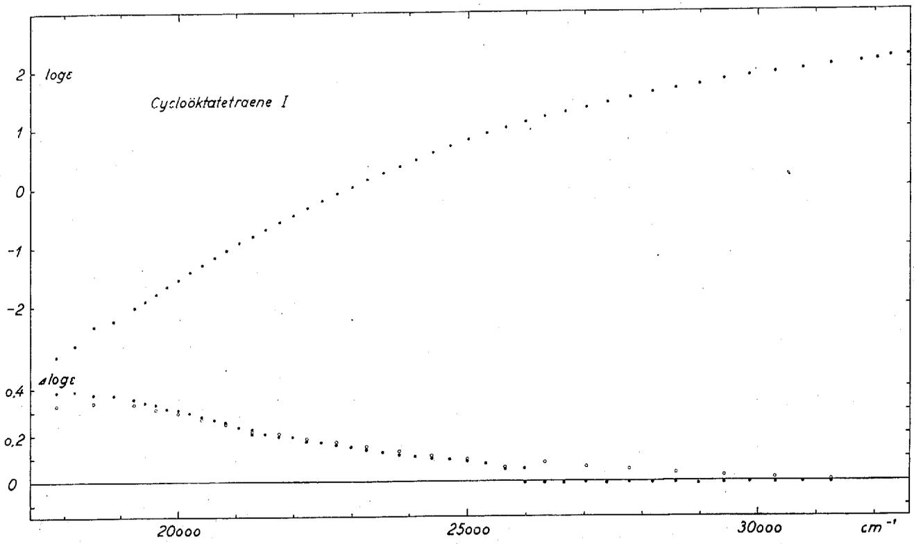
Fig. 26.  $\log \epsilon$  (25°C) and  $\Delta \log \epsilon$  for cycloöktatetraene dissolved in decaline. Because of the instability of cycloöktatetraene the measurements at 25°C were repeated after those at the high temperature. The corresponding  $\Delta \log \epsilon$  are indicated by open circles.
