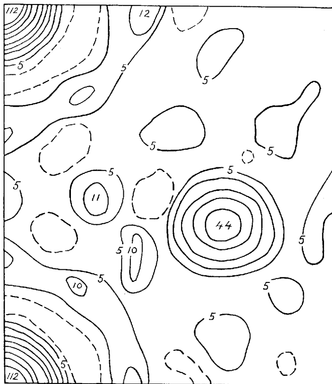
Fig. 6. Projection on 11\bar{2}0 plane from calculated F values for an arrangement of \text{SrCl}_2 with Sr at 000 , Cl at \frac{1}{2}, \frac{2}{3}, 0.42 and \frac{2}{3}, \frac{1}{3}, 0.58 .
