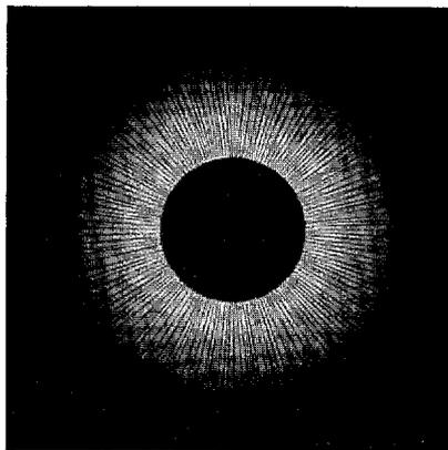
Fig. 7. Pure Negative Figure in Air.
