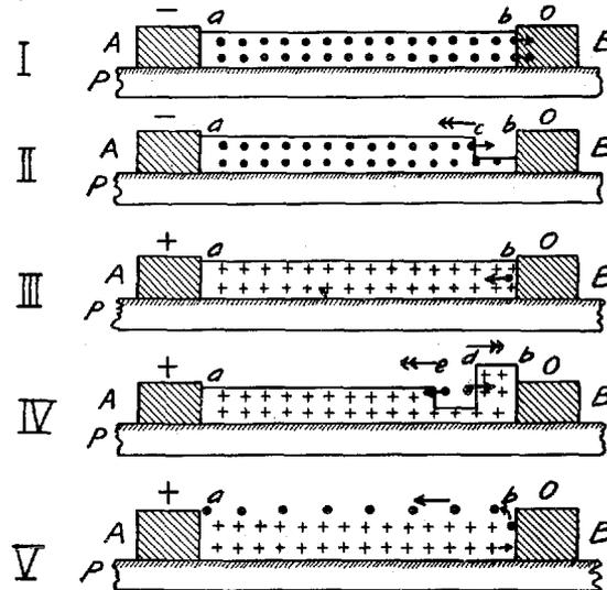
Fig. 29. Schematic Representation of the Conductivity of Negative Figures (I—II) and of Positive Figures (III—IV).
