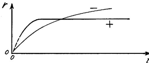
Fig. 21. Schematical representation of the range  $r$  of positive and negative figures as functions of the duration  $t$  of the  $p. d.$
