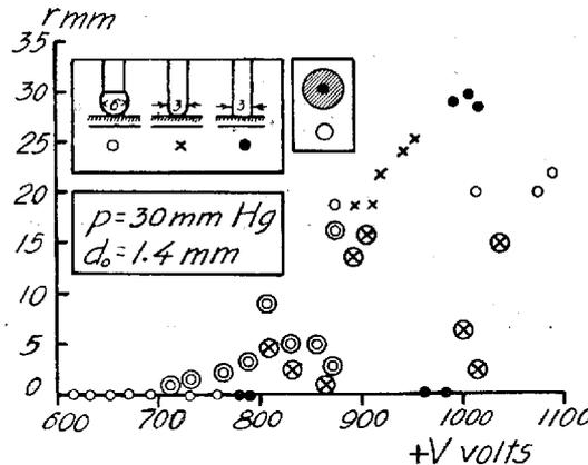
Fig. 13. Range  $r$  as function of the  $p.d.$   $V$  for three different shapes of the electrode. The large circles indicate that the figure has a continuous disc surrounding the electrode. ( $p = 30$  mm Hg;  $d_0 = 1.4$  mm).
