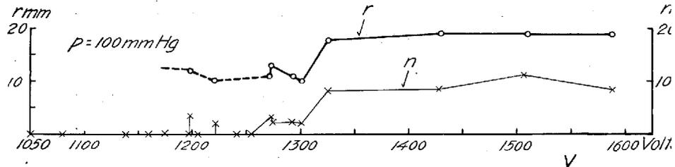
Fig. 12. Range  $r$  and number of spreaders  $n$  as functions of the  $p. d. V.$
