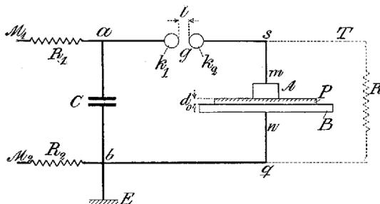
Fig. 1. Diagram of connections for obtaining photographic L. F.  $M_1$  and  $M_2$  are leads from the high tension source.  $R_1$ ,  $R_2$  and  $R_3$  high resistances (slate pencils or the like).  $P$  a photographic plate,  $B$  a metal plate connected to earth  $E$ .
