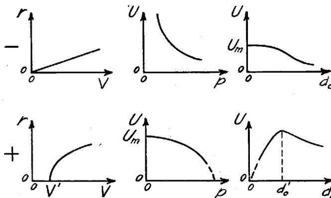
Fig. 8. Schematic representation of (1) the Range  $r$  against the Voltage  $V$ ; (2) the Velocity  $U$  against the Pressure  $p$ ; (3) the Velocity  $U$  against the total Thickness  $d_0$  of the insulating Plate.
