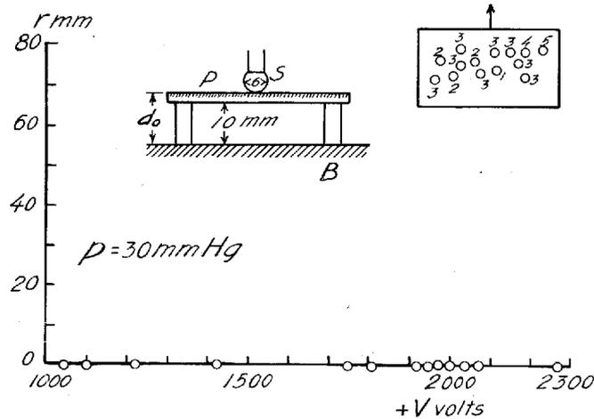
Fig. 17. Range  $r$  of positive figures from a spherical electrode. Thickness  $d_0$  of insulating medium 11.4 mm. Experimental points marked by small circles. The figures at the experimental points denote the number of spreaders.
