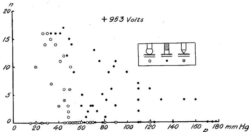
Fig. 16. Number of spreaders  $n$  as function of the pressure  $p$ .
