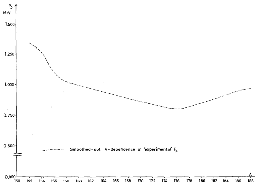
Fig. 6. Average empirical values of the proton odd-even mass difference parameter P_p in region I used in the calculations. This dashed curve is obtained by addition of the smoothed-out (P_p - P_n) -function of fig. 4 to the averaged P_n -values of fig. 1.
