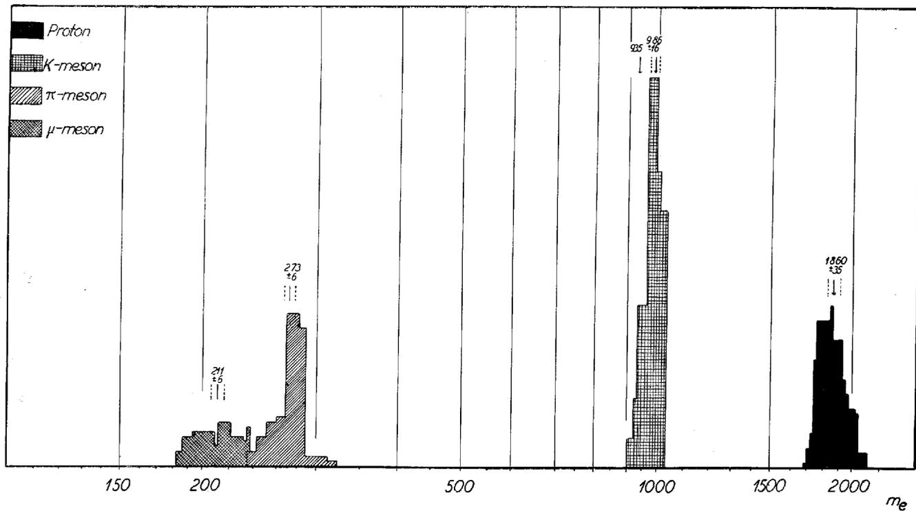
Fig. 2. A weighted distribution (constructed in the same way as Fig. 1) of the masses of the six K-mesons (K 5, K 6, K 7, K 12, K 20, and  $\tau$  2) and the calibration particles, obtained from mean gap-length vs. range measurements.
