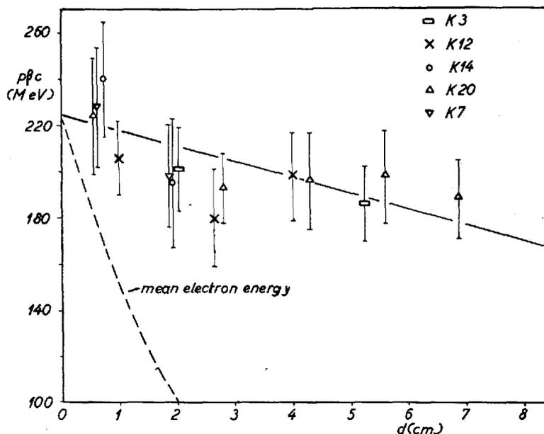
Fig. 4.  $p\beta c$  as a function of the distance from the decay point, for the secondary particles. The full line, corresponding to ordinary ionization loss alone, fits the observations well. The dotted curve, based on the assumption that the secondaries are electrons, and taking energy loss by "bremsstrahlung" into account, is much too steep.
