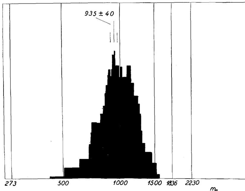
Fig. 1. A weighted distribution of the masses of the 17  $K$ -mesons and one  $\tau$ -meson measured by the constant sagitta method. Each track is represented by a rectangle whose width is the standard deviation, and whose area corresponds to the statistical weight.
