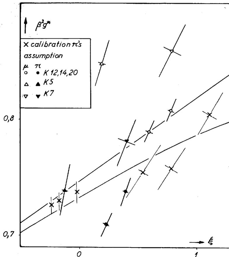
Fig. 3.  $\beta^2 g^*$  vs.  $\xi = \ln \frac{\beta^2}{1 - \beta^2} - \beta^2$  for the  $K$ -meson secondaries and  $\pi$ -meson calibration tracks. Each secondary particle is represented by two points; one calculated on the assumption that the secondary is a  $\pi$ -meson and the other on the assumption that it is a  $\mu$ -meson. The curves represent what are believed to be limiting forms of the theoretical relationship (cf. Appendix). They are fitted at the low energy calibration points.
