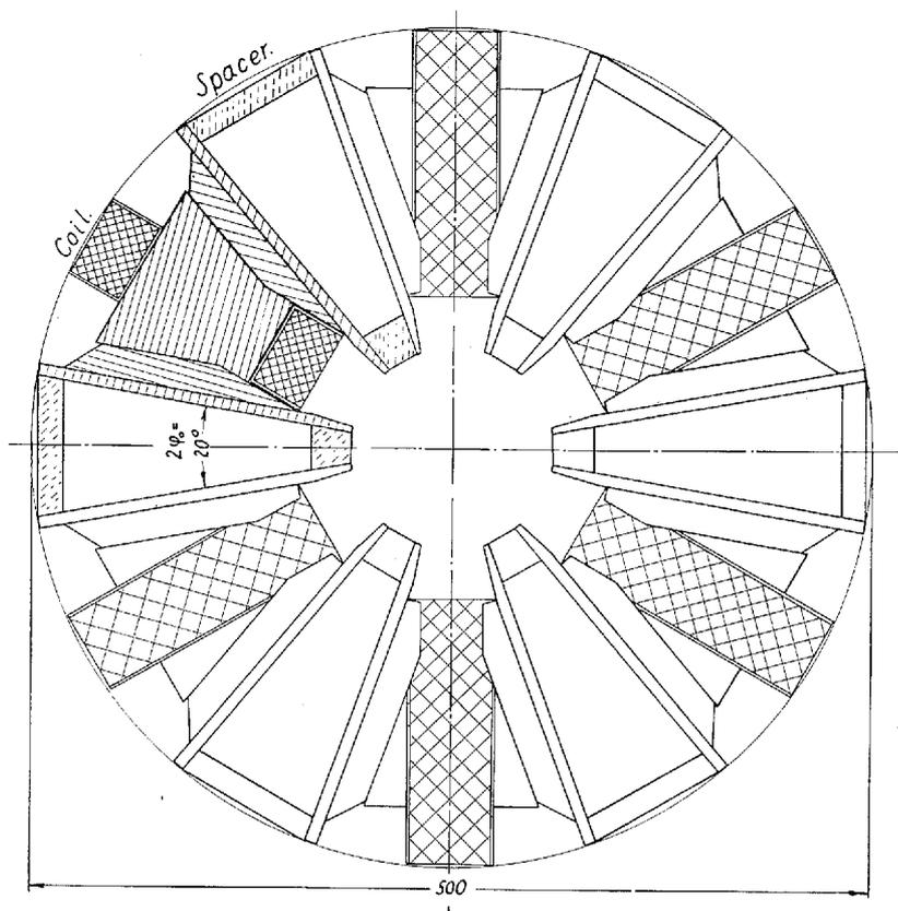
Fig. 1b. Horizontal section through the spectrometer.
