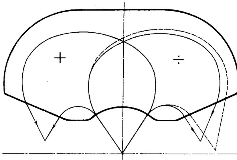
Fig. 10. Pole shape for proposed pair spectrometer.
