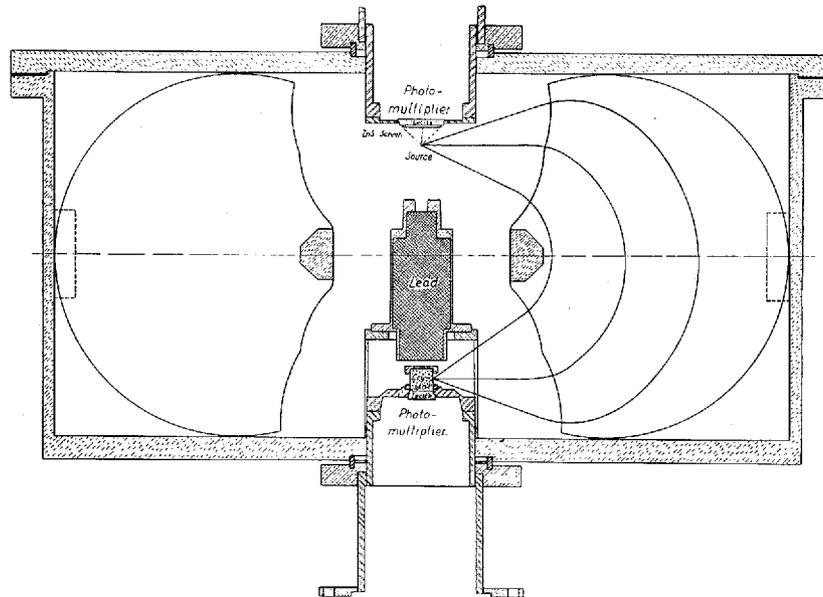
Fig. 1a. Vertical section through the spectrometer.
