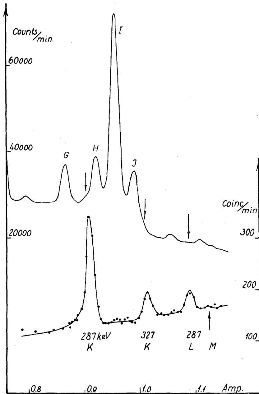
Fig. 9. Above: A part of the complex  $\beta$ -spectrum of  $Th(B + C + C')$ . The lines are given with the notation of Ellis. — Below: The corresponding  $\alpha$ - $\beta$  coincidence spectrum. Random coincidences subtracted.
