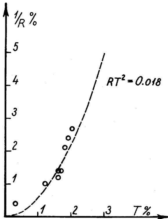
Fig. 8. Transmission versus resolution.
