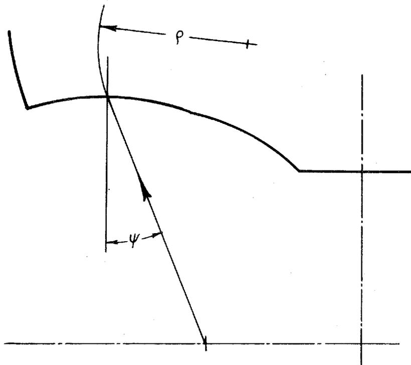
Fig. 2. Entrance of  $\beta$ -ray into the magnetic field.
