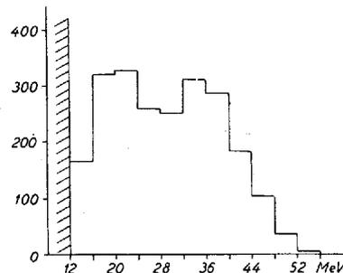
Fig. 7. Energy distribution of fission fragments having traversed 0.93 mg. per cm<sup>2</sup>. of mica.
