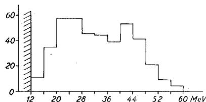
Fig. 9. Energy distribution of fission fragments having traversed 0.73 mg. per cm.<sup>2</sup> of mica.
