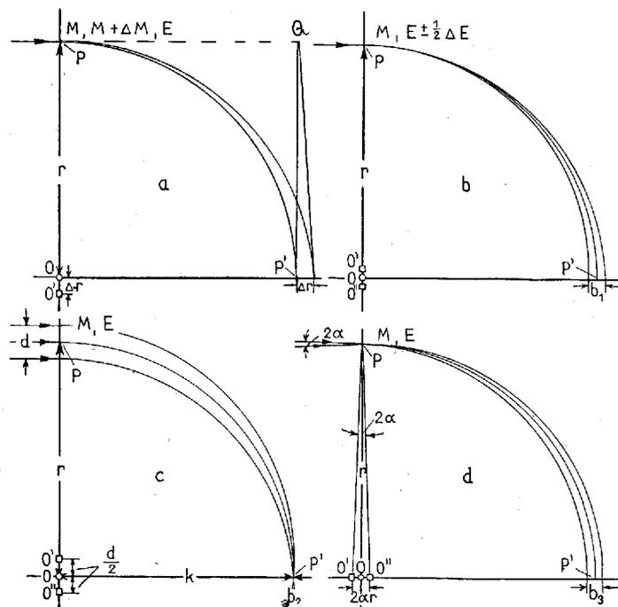
Fig. 2. Ion beams in a homogeneous magnetic field. Ions of mass  $M$  and energy  $eE$  moving on circles with radius  $r$ .
