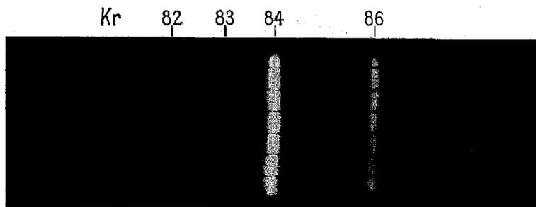
Fig. 11. Mass-spectrum of krypton. Isotopes:  $^{78}\text{Kr}$  (0.42%),  $^{80}\text{Kr}$  (2.45%),  $^{82}\text{Kr}$  (11.79%),  $^{83}\text{Kr}$  (11.79%),  $^{84}\text{Kr}$  (56.85%), and  $^{86}\text{Kr}$  (16.70%).
