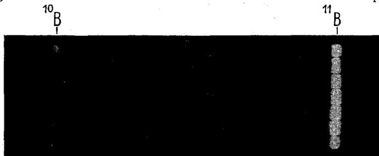
Fig. 8. Mass-spectrum of boron. Isotopes:  $^{10}\text{B}$  (20.6%) and  $^{11}\text{B}$  (79.4%). Photograph of the light from the fluorescent screen. *Leica* camera with *Summitar* objective and *Isopan-Ultra* film. Exposure: ab. 10 sec. Natural size. During the exposure the ion source was supplied with borontrifluoride.
