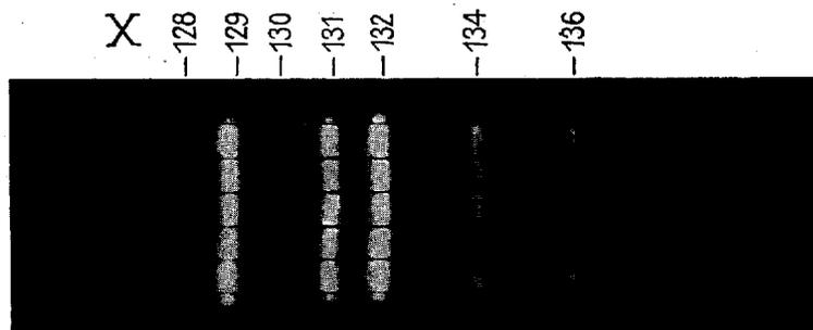
Fig. 12. Mass-spectrum of xenon. Isotopes:  $^{124}\text{X}$  (0.08%),  $^{126}\text{X}$  (0.08%),  $^{128}\text{X}$  (2.30%),  $^{129}\text{X}$  (27.13%),  $^{130}\text{X}$  (4.18%),  $^{131}\text{X}$  (20.67%),  $^{132}\text{X}$  (26.45%),  $^{134}\text{X}$  (10.31%), and  $^{136}\text{X}$  (8.79%).
