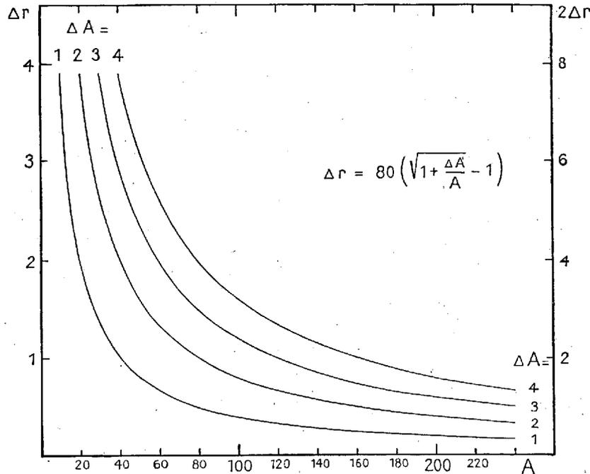
Fig. 3. The mass-dispersion  $\Delta r$  (in cm.) of an ion beam after deflection of  $90^\circ$  in a homogeneous magnetic field as a function of the mass-number  $A$  with  $\Delta A$  as parameter ( $r = 80$  cm.).
